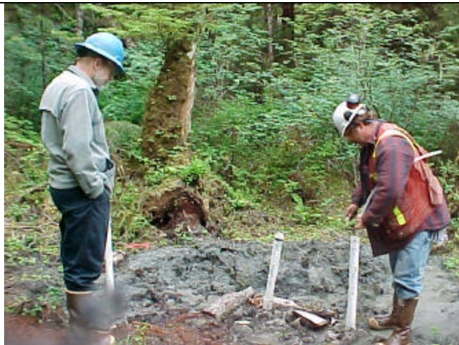
Figure 2. Nested ground water monitoring station located to the west of the tailings facility.
