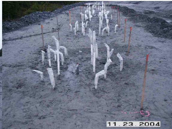
SRMP – lysimeters and sample ports
