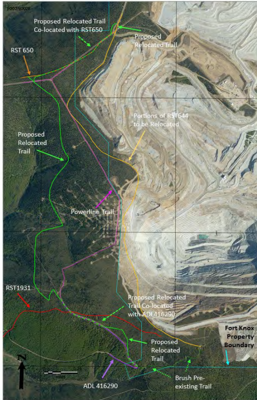
Figure 1-4: RST 644, 650, and 1931 Partial Relocations
