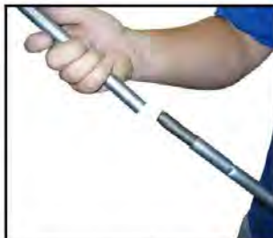
32. Assemble stir rod by inserting upset end over straight end and push together.
