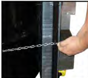
26. Wrap chain around barrel. Pull tight to remove any slack and attach to second hook.
