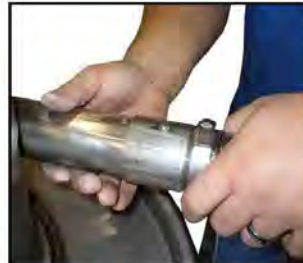
30. Slide flex hose over snap button on 2 inch inlet on drum lid.
