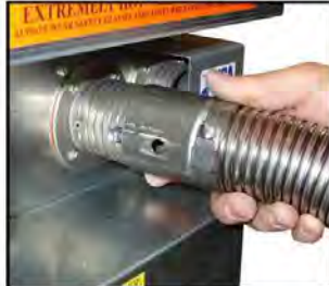
29. Slide flex hose over snap button on 2 inch outlet on plenum.
