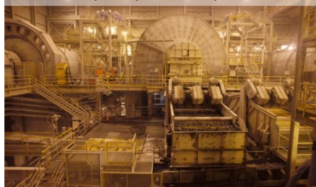
The SAG mill (center) is flanked by two ball mills
