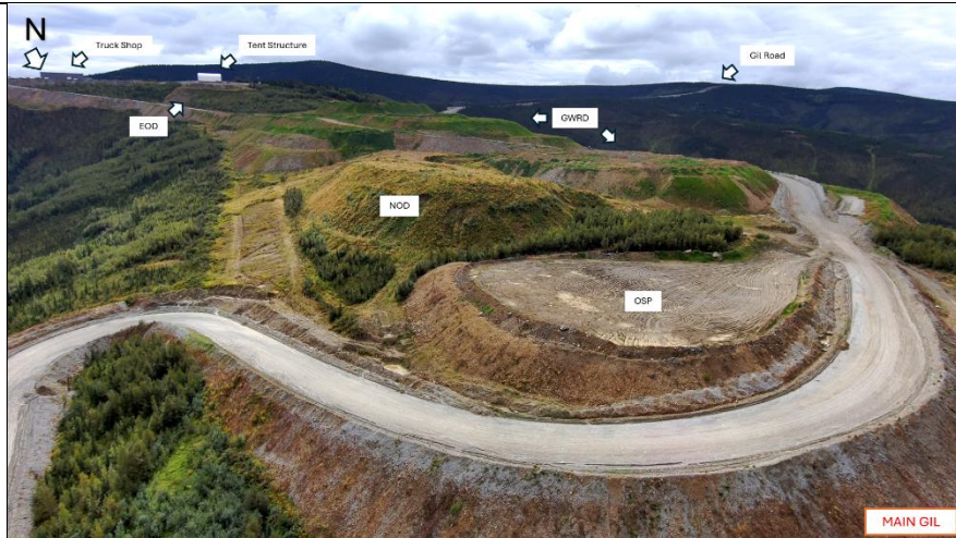
Photo 29: View of Main Gil including truck shop, organic dumps (EOD and NOD), waste rock dumps (GWRD), and OSP.
