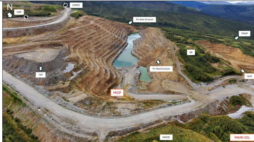
Photo 25: MGP exhibiting areas of pit wall erosion and groundwater inflow.
