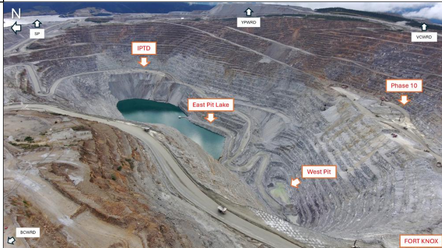
Photo 4: South side of Fort Knox Pit including views of the In-Pit Tailings Disposal , East Pit Lake , West Pit , and Phase 10 drilling and blasting program.
