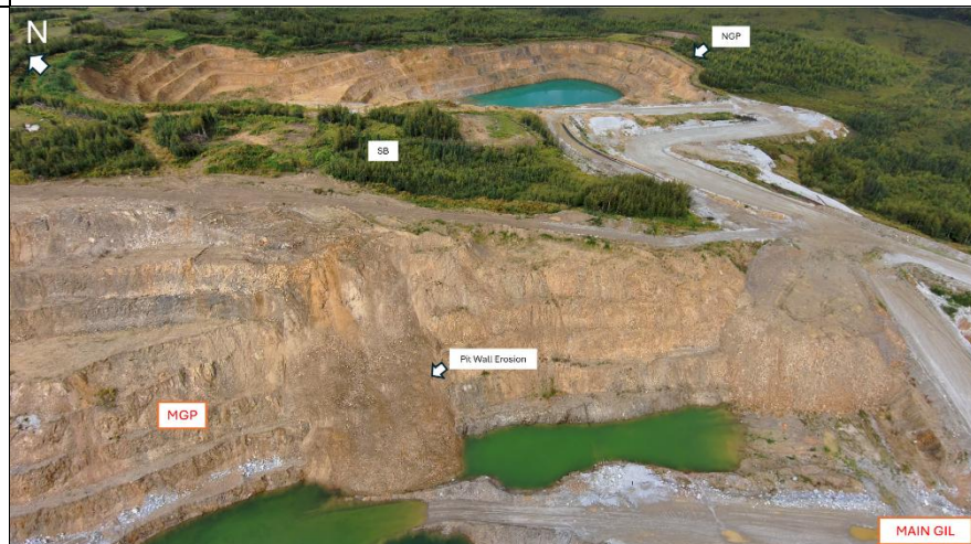
Photo 26: MGP pit wall erosion and groundwater inflow.
