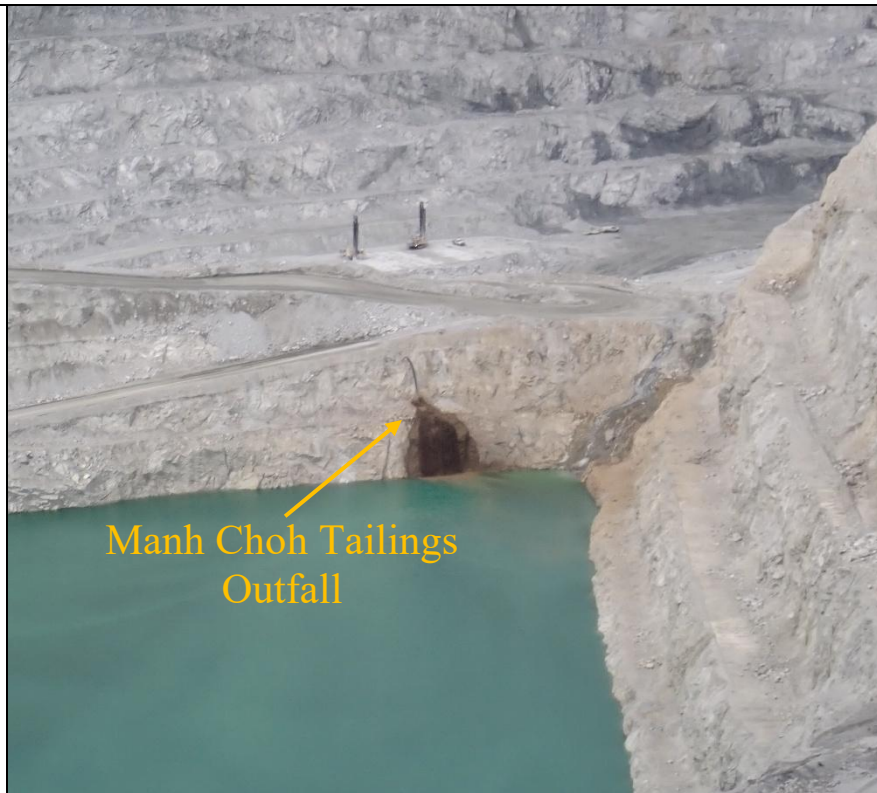
Photo 3: In-pit tailings disposal pond. Active piped tailings discharge into Fort Knox Pit from processing Manh Choh ore.
