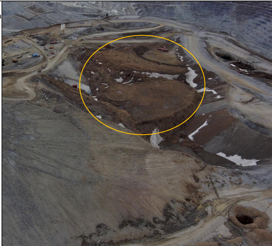
Photo 17: Stockpiled growth media (GM2) at the southern toe of Barnes Creek WRD staged for reclamation.
