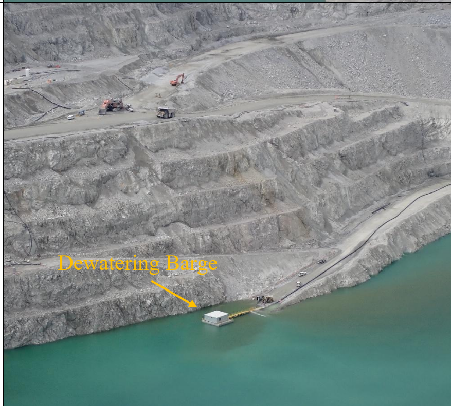
Photo 4: In pit dewatering barge was inactive while tailings were being deposited.
