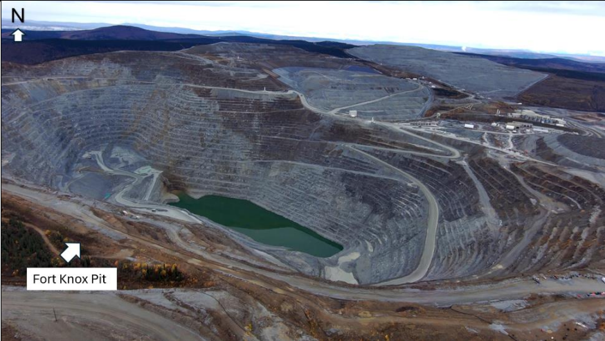
Photo 9: View of the Fort Knox Pit from the top of YPWRD . The outfall and tailings infill of the pit is increasing in depth. BCHL , BCWRD , and WCHL in background.
