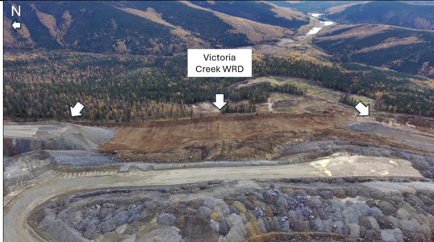
Photo 21: East view of Victoria Creek Waste Rock Dump (VCWRD) including cleared ground and areas of deposition. Confluence of Victoria and Johnson creeks and placer operation in the background.
