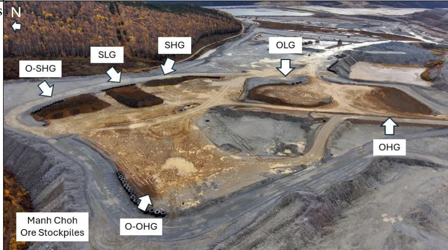
Photo 12: MCOS includes the following: Stockpile 6 Overflow OHG-Oxide High Grade, Stockpile 5 Overflow SHG-Sulfide High Grade, Stockpile 4 SLG Sulfide Low Grade, Stockpile 3 SHG-Sulfide High Grade, Stockpile 2 OLG-Oxide Low Grade, and Stockpile 1 OHG-Oxide High Grade.
