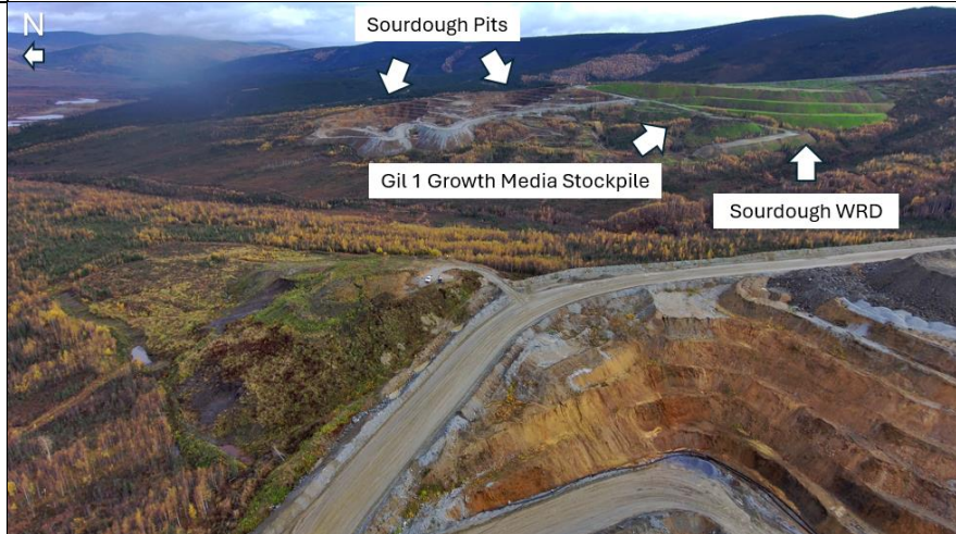
Photo 34: View of Sourdough Ridge from drone above Main Gil Pit. Note hydroseeding taking hold on the SWRD.
