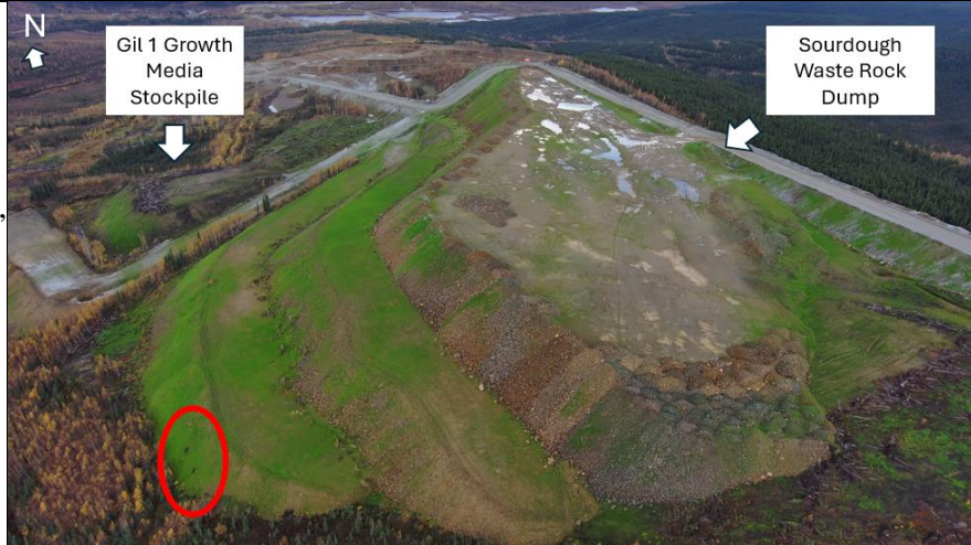
Photo 35: Sourdough Waste Rock Dump (SWRD) and Gil Growth Media Stockpile #1. Hydroseeding is well established on the SWRD, and GM #1, There are two moose grazing on the new growth (bottom left of the SWRD within red circle).
