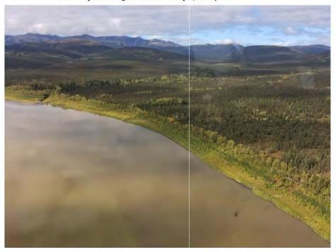
A short bluff up to 16 ft. (5 m) high rises immediately from the shoreline of the Kuskokwim River to a bench that then slopes up at an ~2% away from the bluff. A minimal amount of onshore grading would be required. Surface vegetation and organic surface soils would be removed and piled to the north of the site at the designated soil stockpile location as shown in Figure 3-1.
