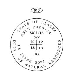
Set 3-1/4" Aluminum Cap On a 30" x 2-1/2" Aluminum Flare End Post, 0.6' AGL; Metallic Gray Cow Magnet Set Under Monument: Carsonite Post 1' North < Set 4" Spruce B.T. bears N81°E, 30.6' < Set 4" Spruce B.T. bears S45°W, 18.9' < Set 6" Spruce B.T. bears N2°W, 28.1'
