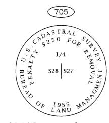
Found 3-1/4" Brass Cap lying next to 2-1/2" Post, 0.1' BGL, Cap buried next to Post < Set 2" Al. Cap on 5/8" rebar bears N29°W, 103.0' < Set 2" Al. Cap on 5/8" rebar bears N61°E, 102.7' < Set 2" Al. Cap on 5/8" rebar bears S36°E, 86.2'
