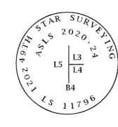
Typical Set Secondary Monument 2" Aluminum Cap On a 30" x 5/8" Rebar ~0.2-0.5' AGL
