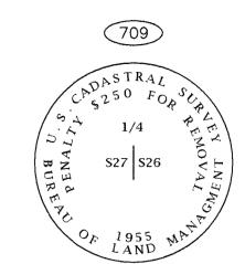
Found 3-1/4" Brass Cap, 0.1' AGL < Set 2" Al. Cap on 5/8" rebar bears S36°W, 86.1' < Set 2" Al. Cap on 5/8" rebar bears N35°W, 86.0'
