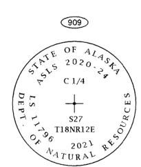
Set 3-1/4" Aluminum Cap On a 30" x 2-1/2" Aluminum Flare End Post, 0.3' BGL; Metallic Gray Cow Magnet Set Under Monument; < Set 2" Al. Cap on 5/8" rebar bears N67°E, 75.3' < Set 2" Al. Cap on 5/8" rebar bears \$23°E, 76.2'
