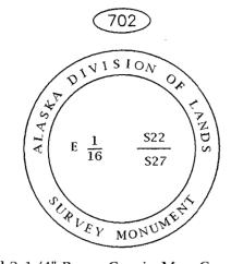
Found 3-1/4" Brass Cap in Mon Case, 0.4' AGL, < Fnd. 6" Spruce B.T. bears N2°E, 53.2' < Set 7" Spruce B.T. bears N58°E, 65.8' < Set 10" Spruce B.T. bears N61°W, 73.8' Cap Markings are Badly Worn
