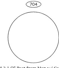
Found 2-1/2" Post from Mon w/ Cap Destroyed, < Set 2" Al. Cap on 5/8" rebar bears N61°W, 103.0' < Set 2" Al. Cap on 5/8" rebar bears N29°E, 102.7' < Set 2" Al. Cap on 5/8" rebar bears N36°E, 86.0'
