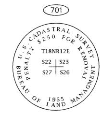
Found 3-1/4" Brass Cap in Mon Case, 0.5' AGL, < Fnd. 13" Spruce B.T. bears N48°W, 53.3' < Set 2" Al. Cap on 5/8" rebar bears \$29°W, 102.9' < Set 2" Al. Cap on 5/8" rebar bears \$61°W, 102.9'
