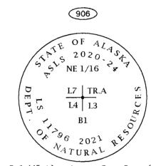
Set 3-1/4" Aluminum Cap On a 30" x 2-1/2" Aluminum Flare End Post, 0.4' AGL; Metallic Gray Cow Magnet Set Under Monument; Carsonite Post 1' North < Set 5" Spruce B.T. bears N69°E, 11.0' < Set 6" Spruce B.T. bears S85°W, 7.3' < Set 5" Spruce B.T. bears N28°W, 10.6'
