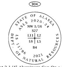
Set 3-1/4" Aluminum Cap On a 30" x 2-1/2" Aluminum Flare End Post, 0.7' AGL; Metallic Gray Cow Magnet Set Under Monument; Carsonite Post 1' North < Set 7" Spruce B.T. bears N29°E, 14.6' < Set 8" Aspen B.T. bears \$36°E, 10.1' < Set 5" Spruce B.T. bears S28°W, 1.1'
