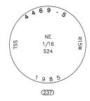
FOUND 2-1/2" ALUM. CAP, ON ALUM. POST WITH FLANGES BROKEN OFF, IN A DISTURBED CONDITION; NOT USED AS THE POSITION FOR THE CORNER POINT.
