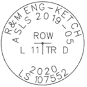
SET 5/8" X 30" LONG REBAR (UNLESS OTHERWISE NOTED) AND 2" ALUMINUM CAP WITH PLASTIC INSERT
