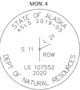
TYPICAL SET 2.5" DIA. X 30" ALUM POST MON. WITH 3.25" DIA. ALUM. CAP. A METALLIC GRAY COW MAGNET IS BURIED AT THE BASE OF THE MON. AND A CARSONITE WITNESS POST IS SET 1' NORTH OF MON.
