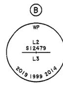
Found a stainless steel post, 2 1/2 in. diam., firmly set, flush with ground, with brass cap mkd. WP L2 S12479 1999 2014, from which the original bearing trees
