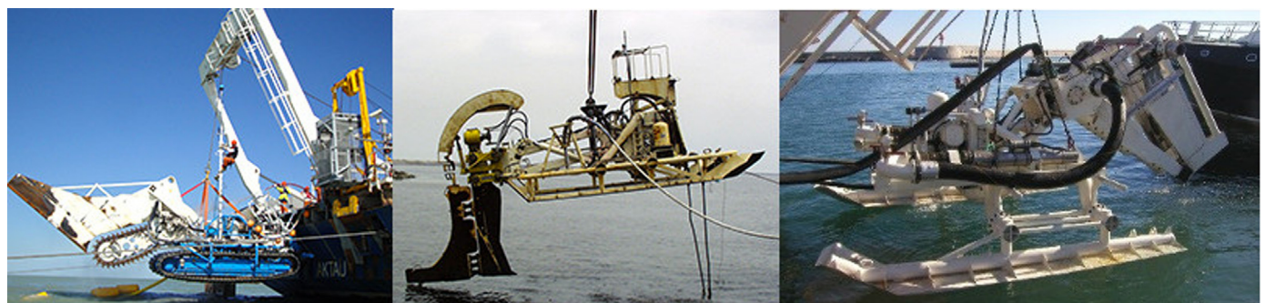
Fig. 1. Wheel cutter (left); Plough (centre) and Towed Jetting Vehicle (right) (courtesy: www.ldravocean.com).
