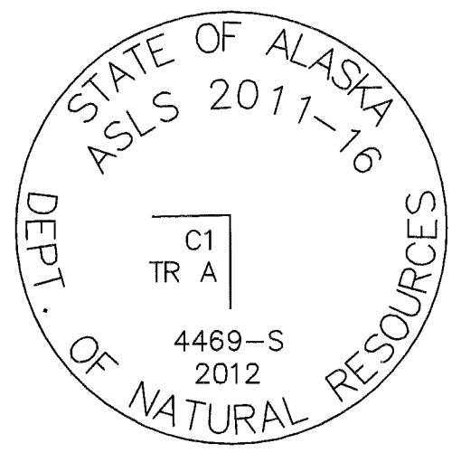
3-1/4" aluminum cap on 2" I.D. x 30" aluminum pipe, 0.2" above ground.
