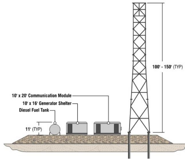
**Figure 2-4. Typical communication site layout**
