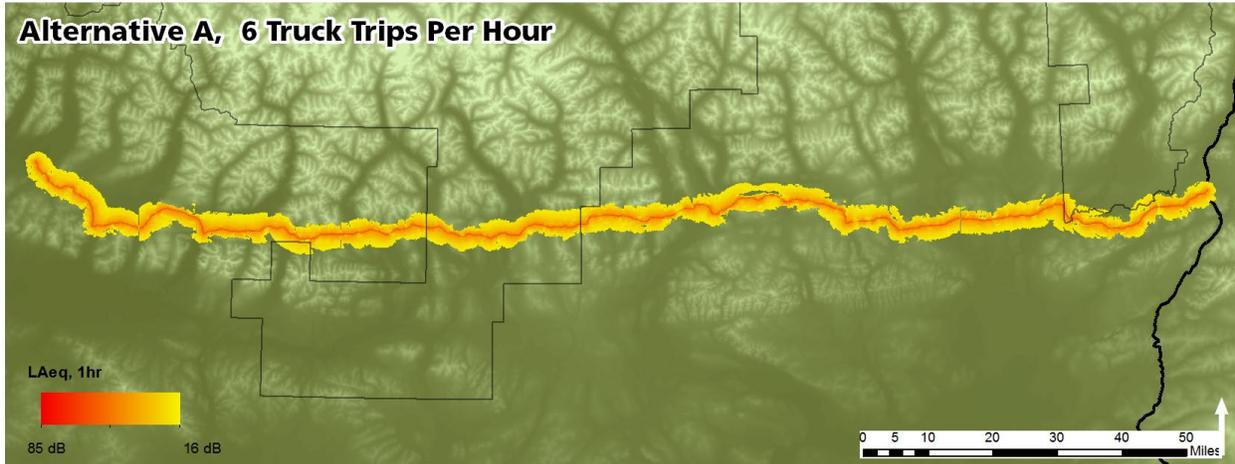
Figure 2. Modeled LAeq, 1hr for Alternative A given 6 truck trips per hour at 45 mph. Data are clipped to an ambient LA90 of 16 dB.
