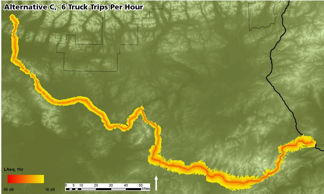
**Figure 4. Modeled LA<sub>eq</sub>, 1hr for Alternative C given 6 truck trips per hour at 45 mph. Data are clipped to an ambient LA<sub>90</sub> of 16 dB.**
