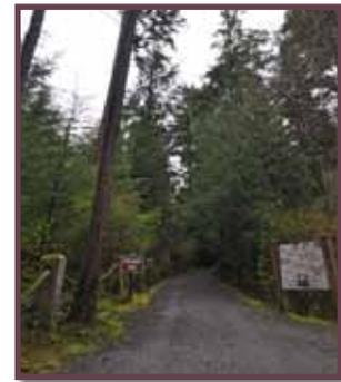
**TOTEM POLE LOOP TRAIL:** The segments of this trail leading past the clan house and to the board walks are also accessible and in good condition. The trail segment on the northern end of the open grassy area has an average slope of 6.0% and is too steep for wheel chairs according to ADA standards. This trail segment is part of the original trail system.
