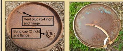
Figure 3. Typical tight-head drum with closures (left), and open (removable) head with lever closure (right).
