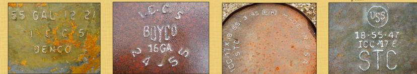
Figure 6. Base marks exhibiting manufacturer and ICC regulatory codes (embossing enhanced by chalk).
