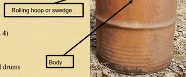
Figure 4. Cylindrical tight head drum body.
