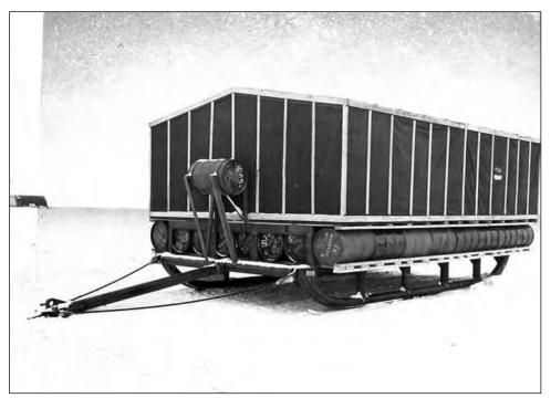
Figure 33. Amphibious food wanigan, located near Barrow, 1950 (Source: U.S. Geological Survey Professional Paper 301, Figure 74, 1958).
