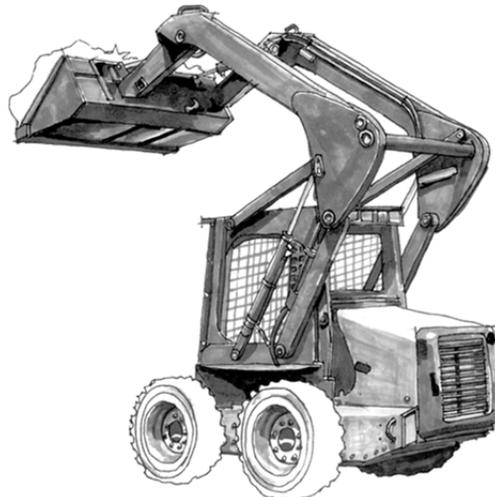
**Figure 6.36 – Skid-Steer Loader**
