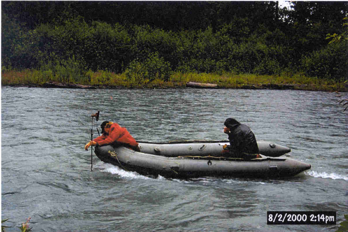
Photo 3: Discharge measurement under higher flow conditions using a boat.
