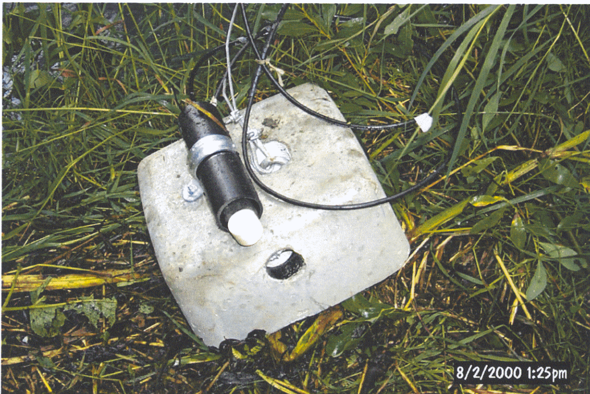
Photo 2: Sensor block with pressure transducer and conductivity probe.
