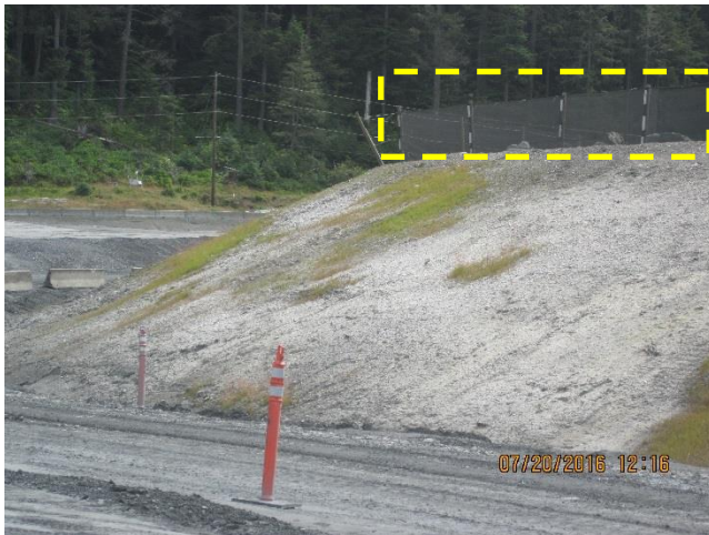
Photo 18. A portable windscreen highlighted in image is used for reducing tailings dust dispersal.
