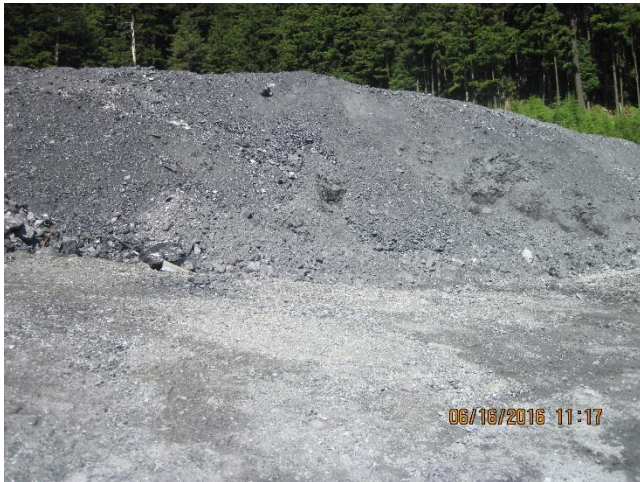
Photo 16. Site 23 Class 1 (Argillite) waste rock.
