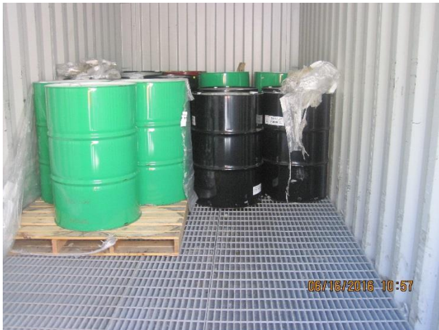
Photo 8. Storage containers are tidy and with secondary containment.
