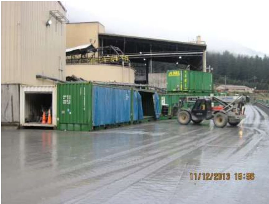
Photo 13. The drums and tote of used oil products were temporarily placed in this sea van. The sea van is on a concrete surface that drains to Pond A.
