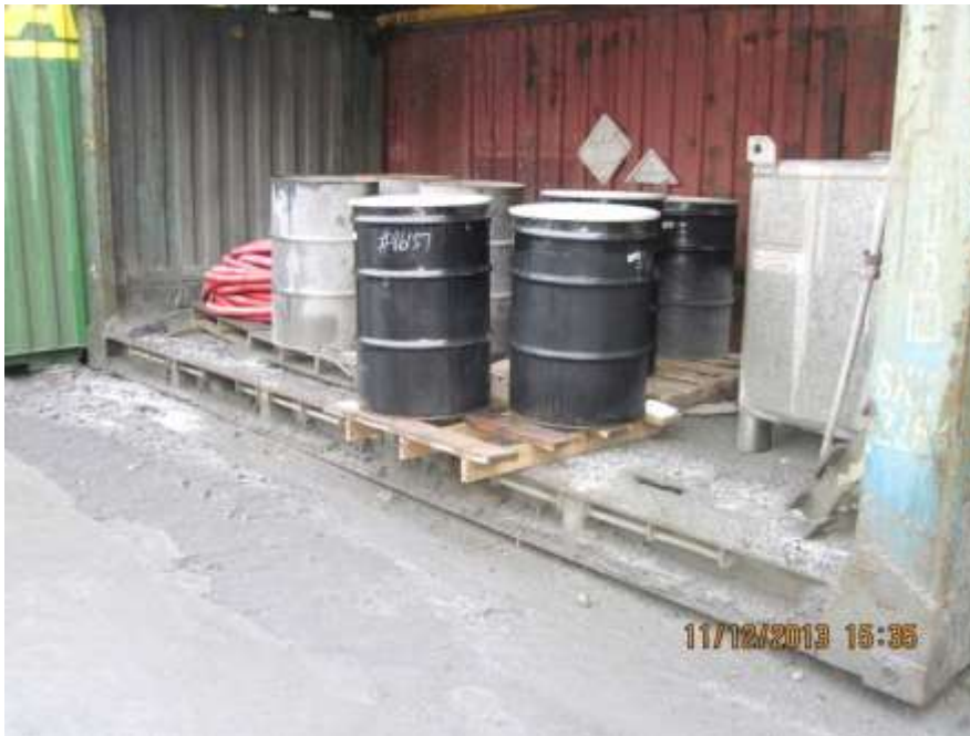
Photo 11. Several drums and a tote of used petroleum products were stored at the Used Petrol Conex. There is no secondary containment and the conex is not on concrete that drains to Pond A.
