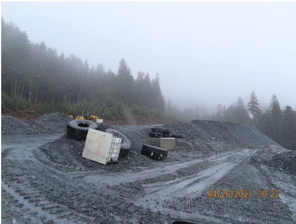
Photo 8. Site 23. Class 1 waste rock is separately stored from Class 2/3 waste rock.
