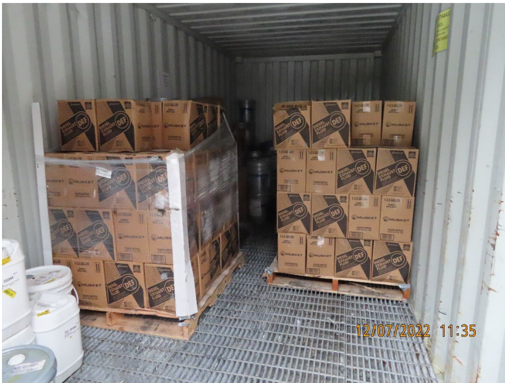
Photo 5. Chemicals stored in appropriate secondary containment at the 920 warehouse area.
