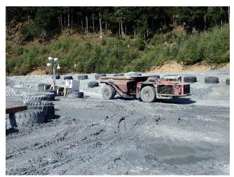
Photo 6. A haul truck depositing class 2 and 3 waste rock at Site 23.
