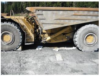
Photo 7. A haul truck with a couple of fluid leaks.
