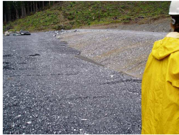
Class I argillite (left), Class II phyllite (right)
