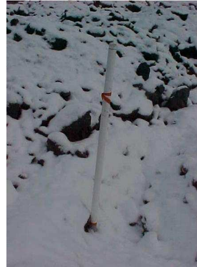
Monitoring Device Without Lock
