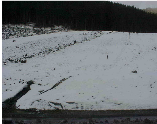
Production Rock Site 23 - Final Cover Test Plot Showing Exposure At Sides To Air
