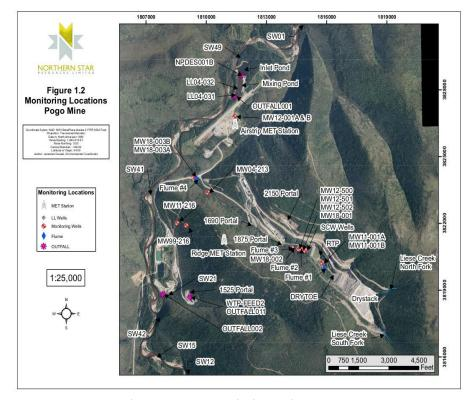
Figure 1.2: Water Monitoring Stations
