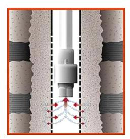
Figure 17.1.1: Cross Section of Waterra® Foot Valve
