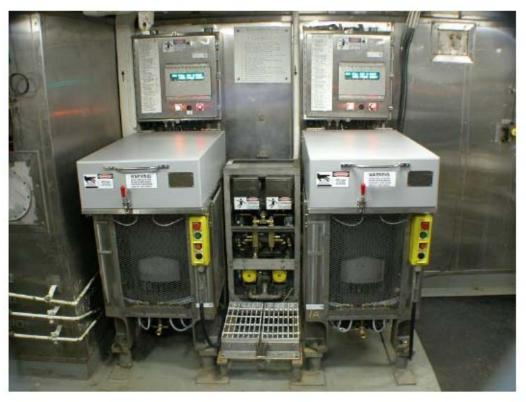
The U.S. Navy's Plastics Waste Processor converts shipboard-generated plastic waste into a dense, sanitary disk suitable for long-term storage. This waste stream includes lightly food-contaminated as well as clean plastic. The Plastics Waste Processor is designed to handle other materials that may be combined with, or contain, plastic components that cannot be processed in the normal solid waste stream.
