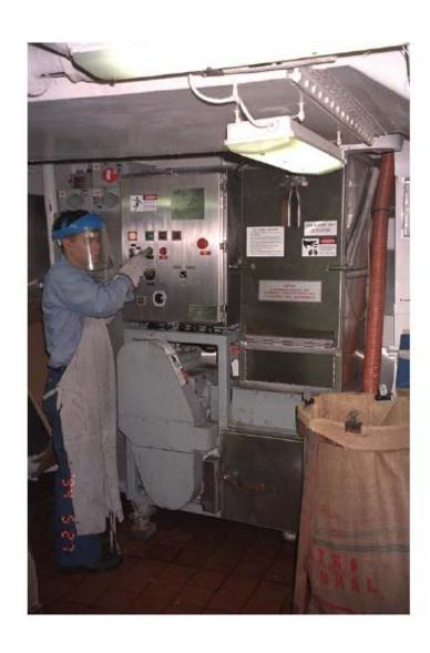
The U.S. Navy developed the Solid Waste Shredder to process shipboard plastics, metal and glass. The Solid Waste Shredder is designated as a Plastics Shredder for plastic waste use, and as a Metal and Glass Shredder for metal and glass.
