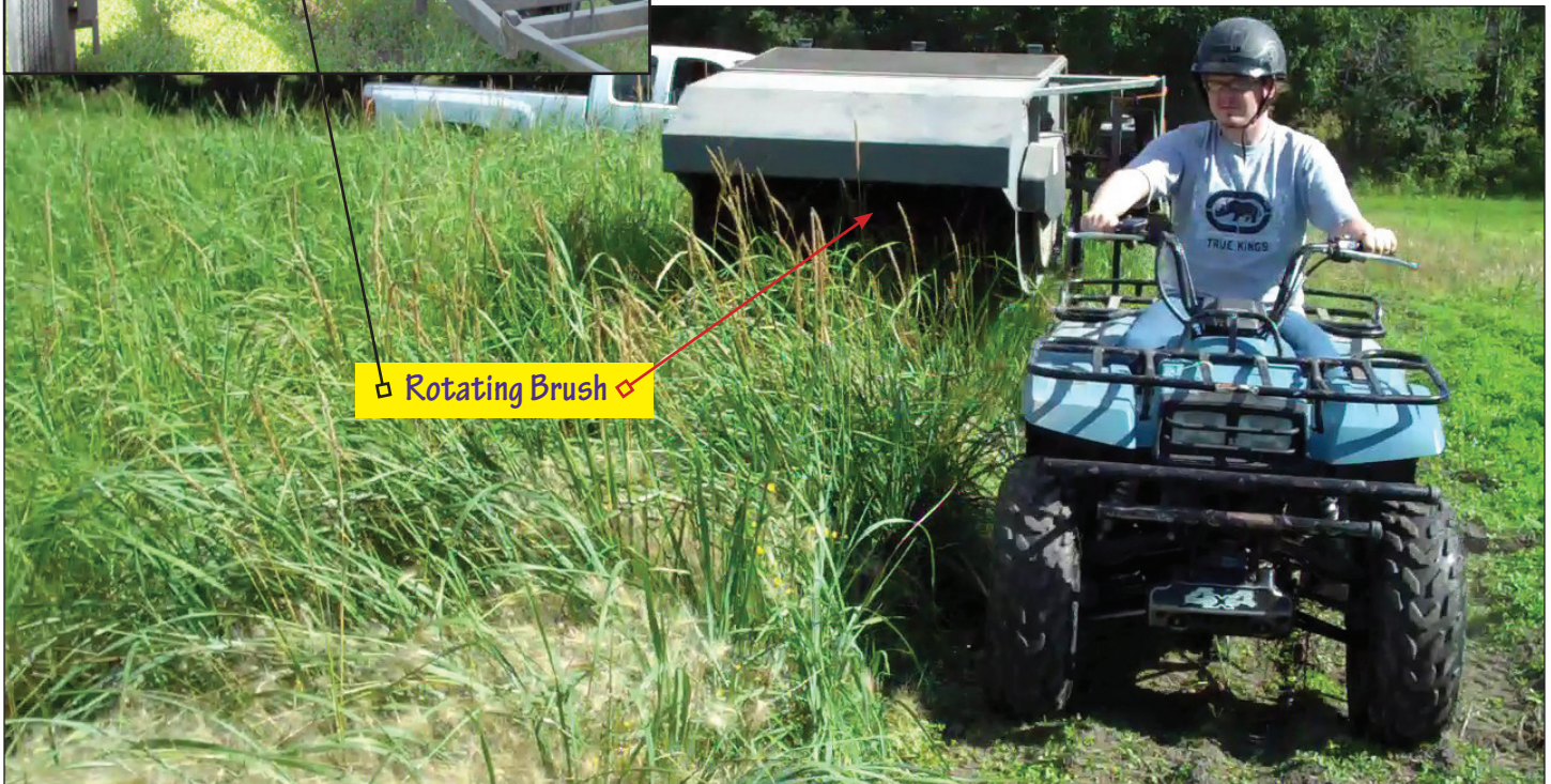
Harvesting with the Seed Stripper
