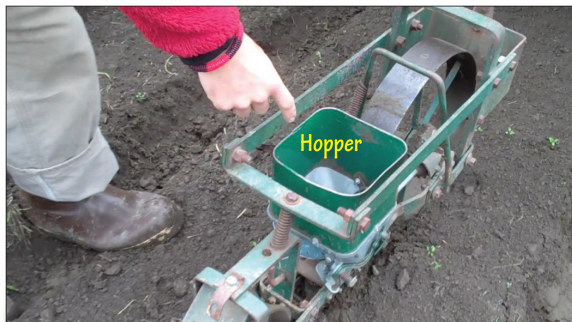
Planting bluegrass in the fields of Alaska Plant Materials Center using Planet Jr.
