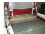
Agropyron violaceum cleaning with an air-screen cleaner
