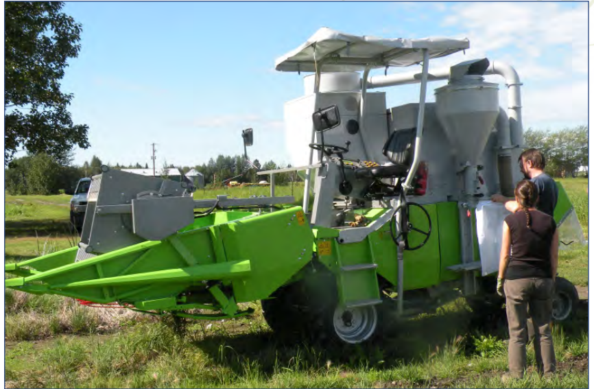
The PMC's Wintersteiger combine conditions seed as it is collected
