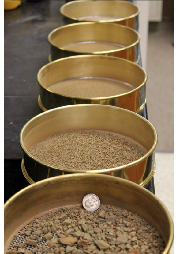
Soil sieves are used to separate a soil profile into constituent parts for analysis.
