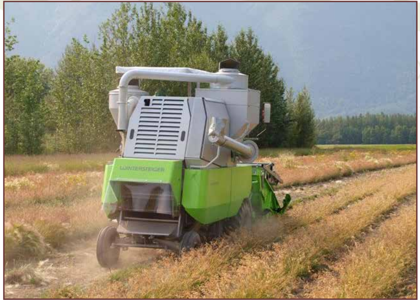
The PMC's Wintersteiger combine conditions seed as it is collected.
