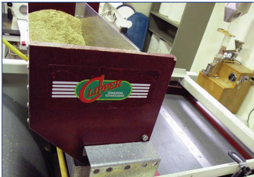
The screen separator uses vibrating screens to separate chaff from target seeds
