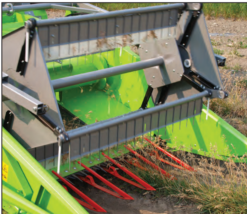
The Wintersteiger combine in use at the PMC performs some basic conditioning of harvested crops, reducing the time required for post-harvest cleaning
