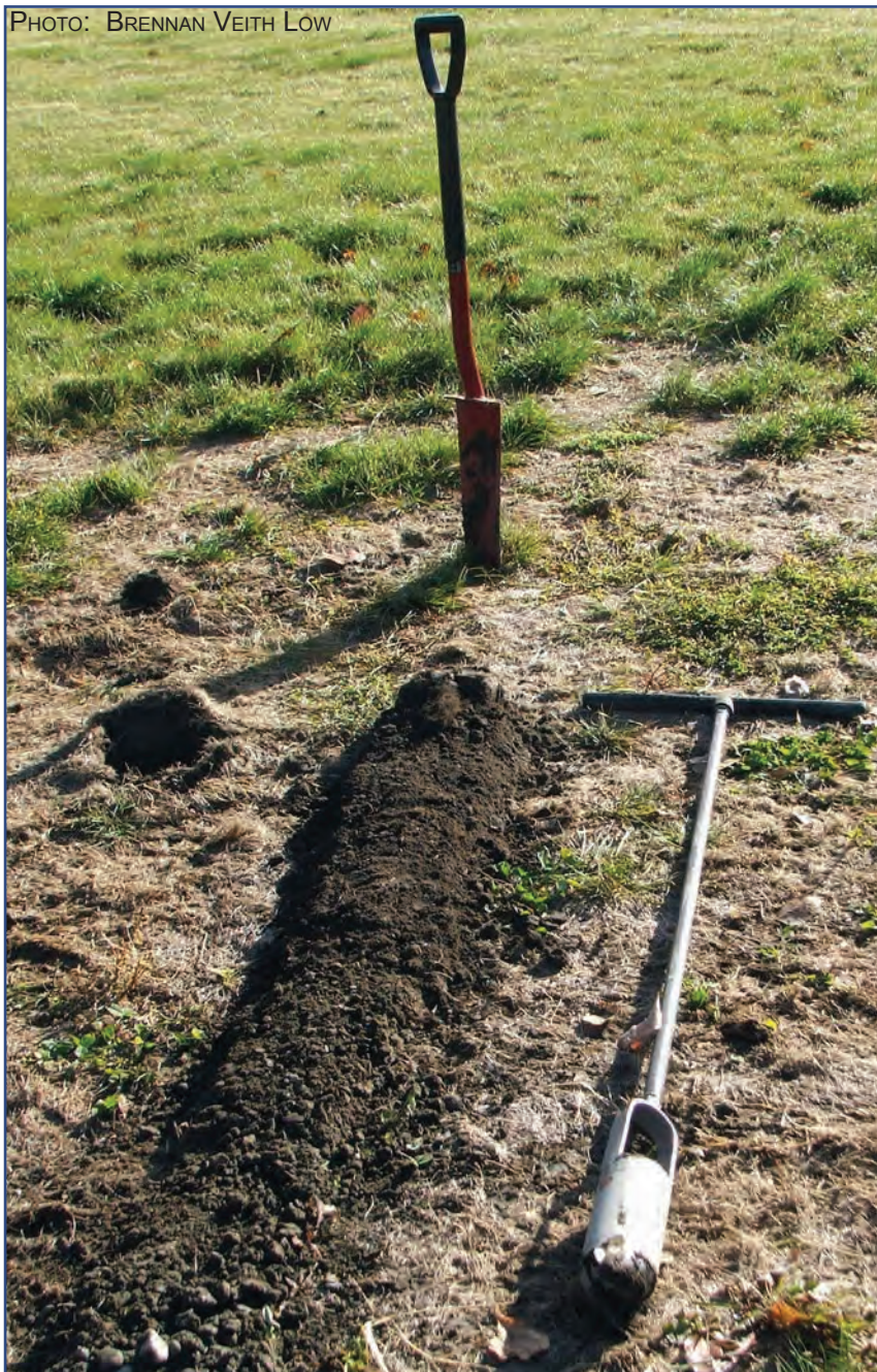
A soil monolith that was extracted using a hand-auger and spade-shovel; tools commonly used to dig a soil horizon. A monolith shows the texture and character of distinct horizons within the soil profile.
