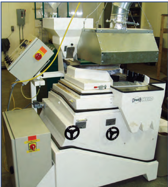
Plant materials of similar size but different densities are separated using a gravity separator
