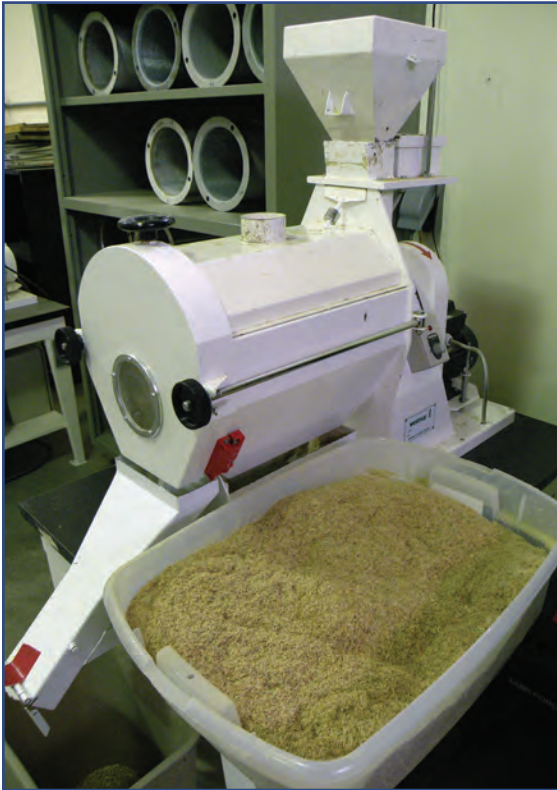
A brush cleaner uses rotating brushes to separate seed from inert plant materials
