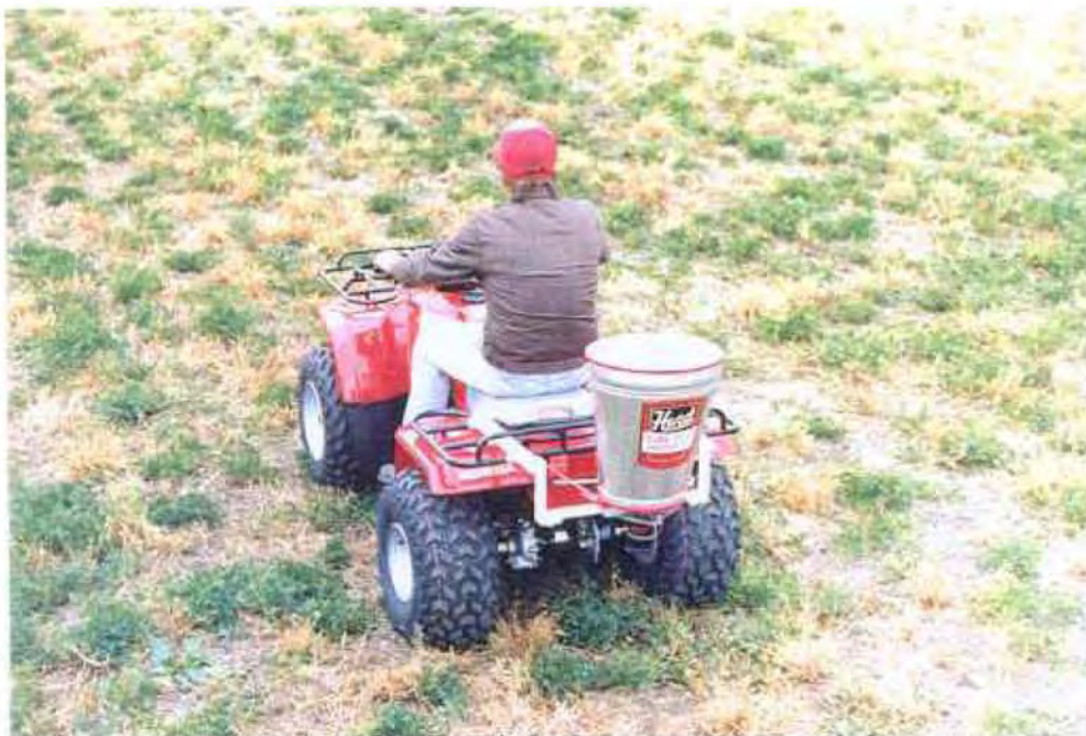
Figure 3.5.2 Spinner Type, Electric Spin Photograph Courtesy of Herd Seeder
