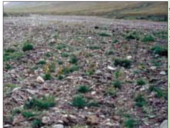
The effect of surface scarification on plant establishment and growth after two growing seasons. No seed was applied to the site, but it was fertilized with 20N-20P-10K at a rate of 500 pounds per acre.
