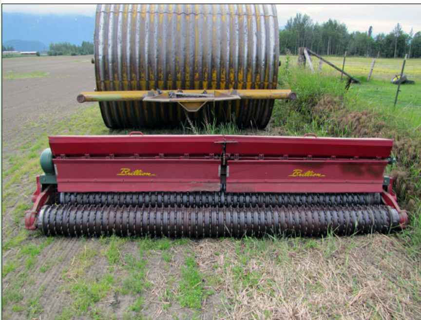
A drill seeder, in this case a Brillion ©, is often used for planting revegetation species. The large drum in the background is an imprinter, used to firm the seedbed as well as create furrows into which the seed will settle.
