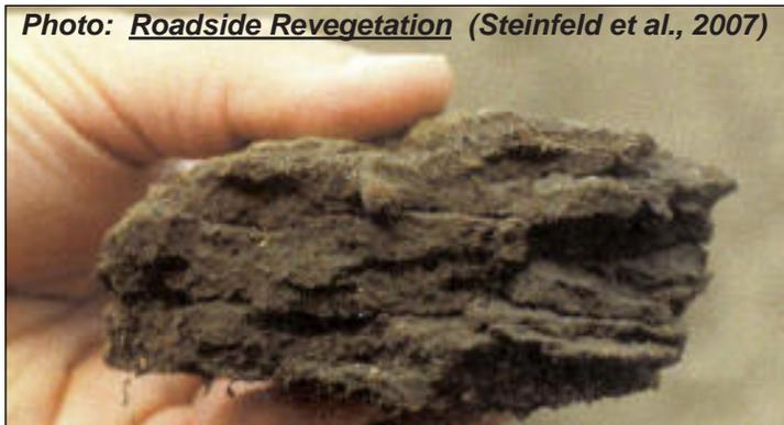
Figure 6: Heavily compacted soil; Note platy structure. Water flow through this soil is poor.
