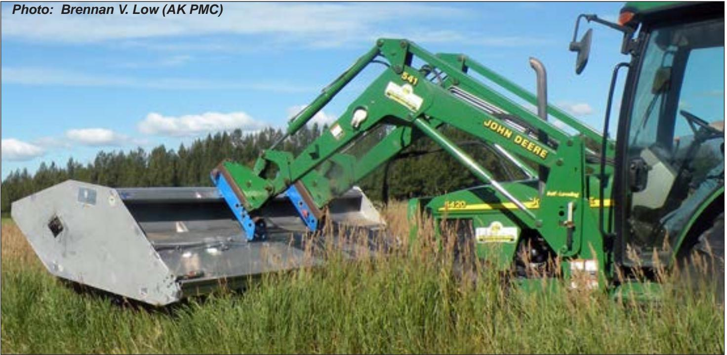
Figure 25: Using a seed stripper leaves the inflorescence (seed-head) intact, allowing for multiple equipment passes previously described, before planting can begin.
