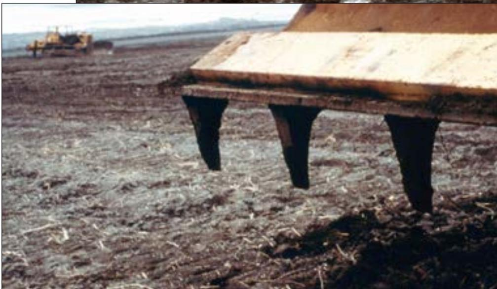
Deep scarification of the soil surface can be accomplished with a grader with a 'ripper shanks' tool bar
