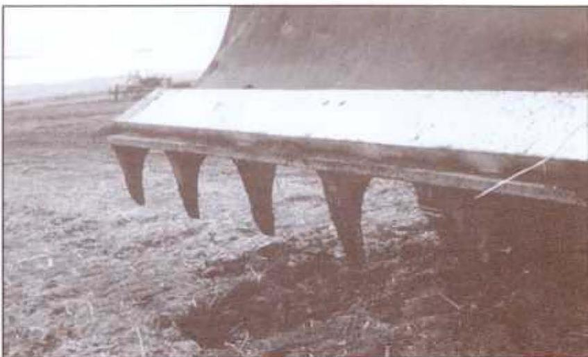
FIGURE 12. *Modified dozer blade with tiger teeth used to prepare site*
