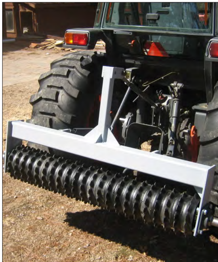
An imprinter can be used to firm sandy, silty or loose soils
