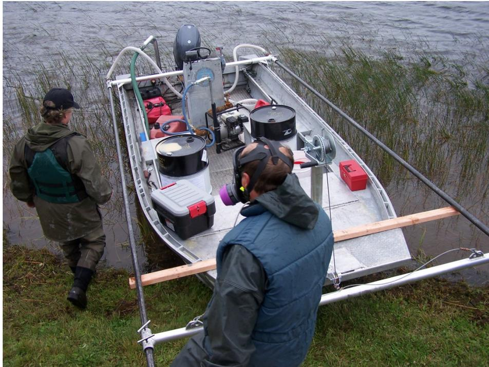
Figure 11. Motorboat and a well-pipe boom system currently used by the Alaska Department of Fish & Game for deep-water application of rotenone. It may be used if Sonar Genesis is applied in mid- to late-summer when thermoclines may develop in Beck and Daniels Lakes.
